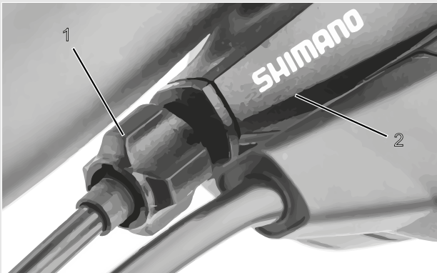
Figure 81: Adjusting sleeve (1) for the single-cable, cable-operated gear shift with shifter housing (2), example
