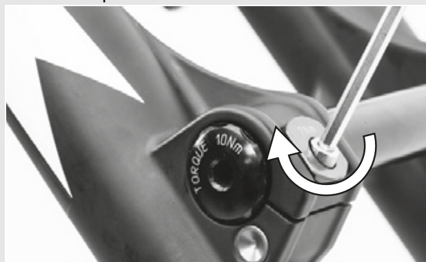
Figure 25: Tightening the securing clip
