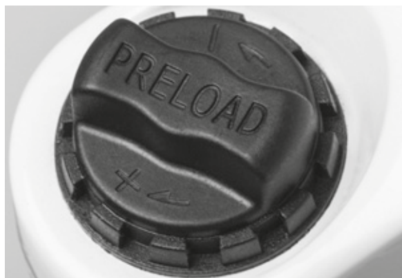
Figure 52: Negative deflection setting wheel on the suspension fork crown
