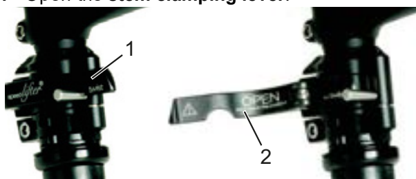
Figure 46: Open (2) and closed (1) stem clamping lever; by.schulz speedlifter used as an example
