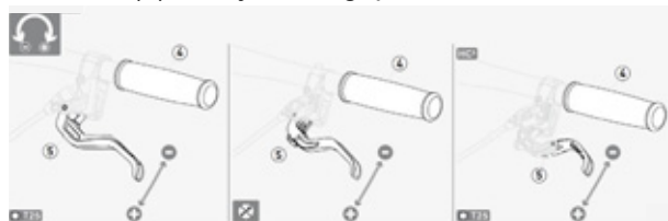
Figure 50: Setting the grip distance on a Magura disc brake lever
