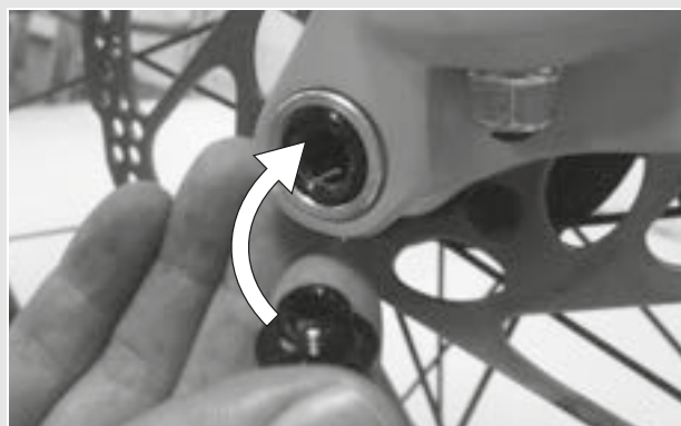
Figure 22: Pushing the quick release lever into the axle
