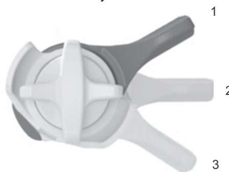
Figure 65: FOX compression adjuster on the rear frame damper with the OPEN (1), MEDIUM (2) and HARD (3) positions
