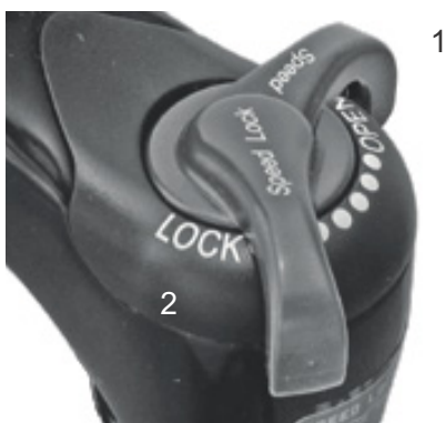
Figure 67: Suntour compression adjuster with the OPEN (1) and LOCK (2) positions
