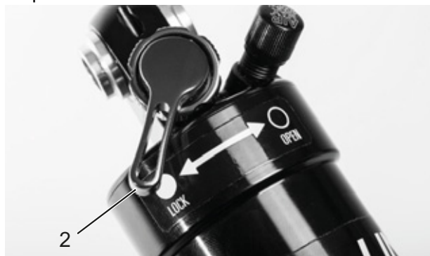
Figure 69: Suntour compression adjuster closed (2)
