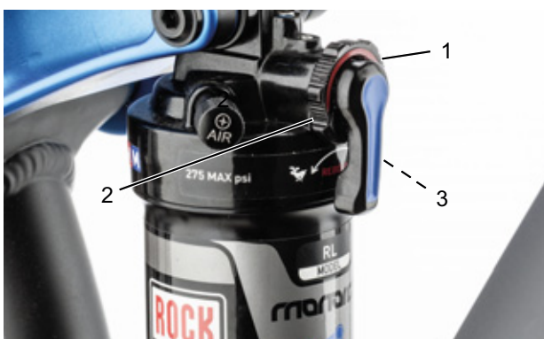
Figure 70: Setting the rebound damper strength on the rear frame damper setting wheel (1)
